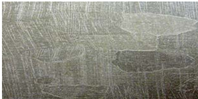
Fig. 1: Grain structure of GOES
